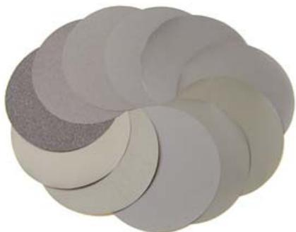
Ultrafine Laboratory Abrasives, manufactured by 3M Company, are a paper backed silicon carbide product. Intended to be used in wet applications, these fixed abrasives are exceptional in extending the fine grinding steps beyond the 600 grit. Graded on the ANSI system, the United States abrasive standard, this product is available in 1000, 1200, 1500, 2000, and 2500 grit. Forms available include discs, sheets and rolls.
